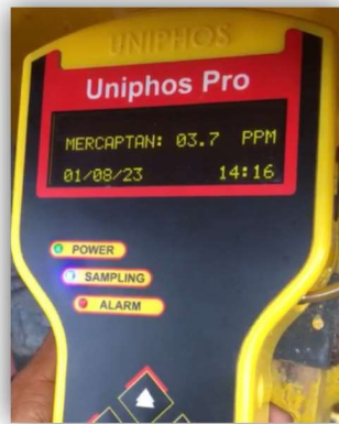
Figure-14: Odourant gas analysis
